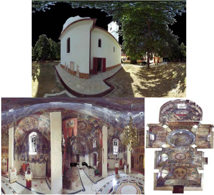
Picture 15. Documentation of the Bođani Monastery, 18th century, made in 3D laser technologies
