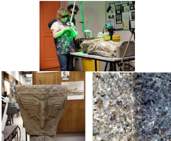
Picture 23. Laser cleaning of stone archaeological artifacts in Central Institute for Conservation in Belgrade- CIK
